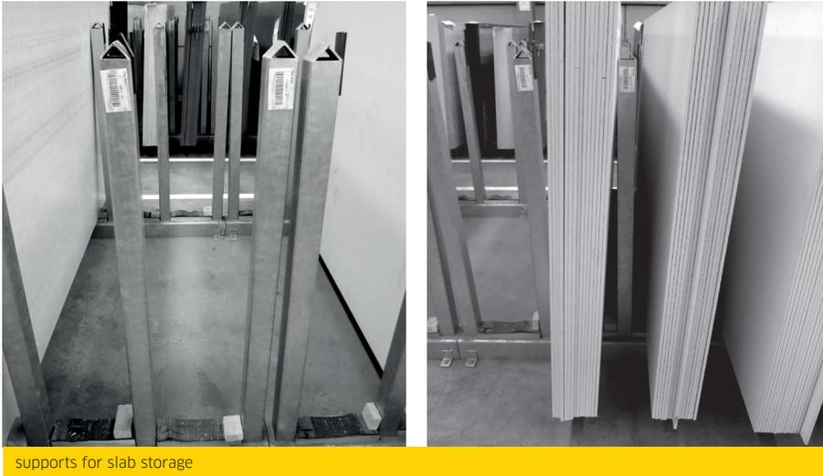
3 mm and 6 mm slabs need at least three support points, distributed evenly along the back of the slab; a full support is recommended - an unused granite or marble slab with sufficient width, for example. The best way to maintain the integrity of the slabs is to keep them in their original packaging or use a full support on the back of the slab such as an unused granite or marble slab which is wide enough.
