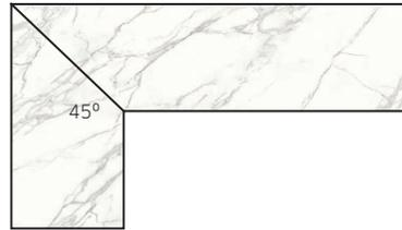
L-shaped countertops made of a single piece without a 45° angle must have a minimum radius of 2”.
