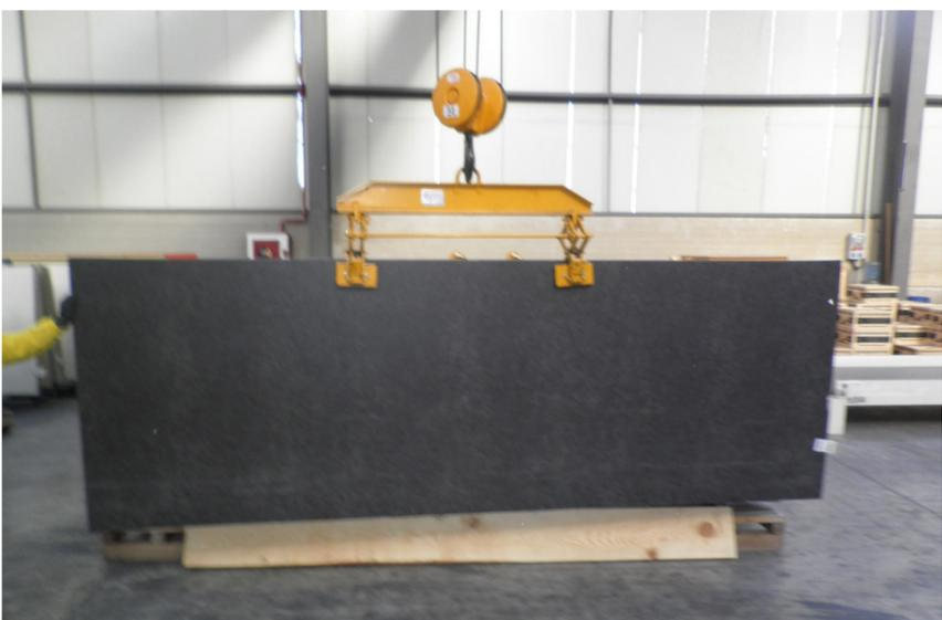
The additional width of the clamp will prevent the slab from bending and twisting when transporting and thus avoiding unwanted ruptures.
