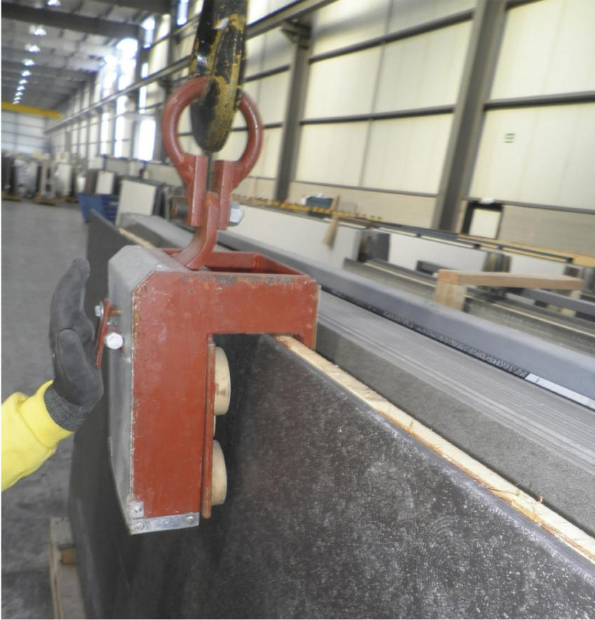
5. Fix the clamp and lift the slab(s) with caution. Try to avoid sudden changes of direction.
