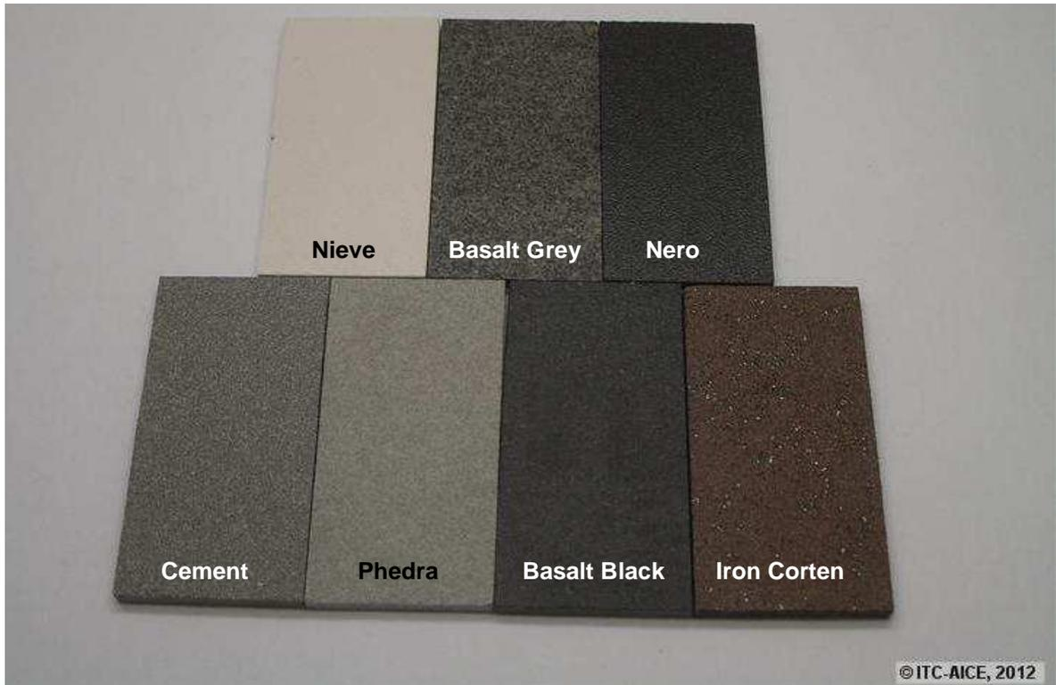
*Figure 3 Appearance of the tiles after 28 days of light exposure.*
