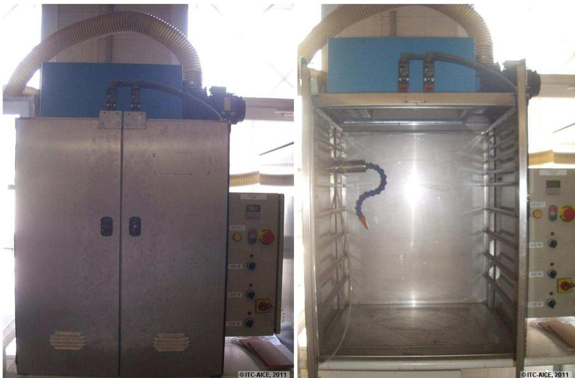
Figure 2 Photographs of the mercury vapour lamp exposure chamber used.
