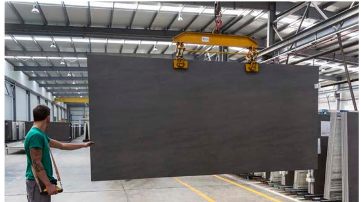
Image 2: Neolith slab handling with Clamp
