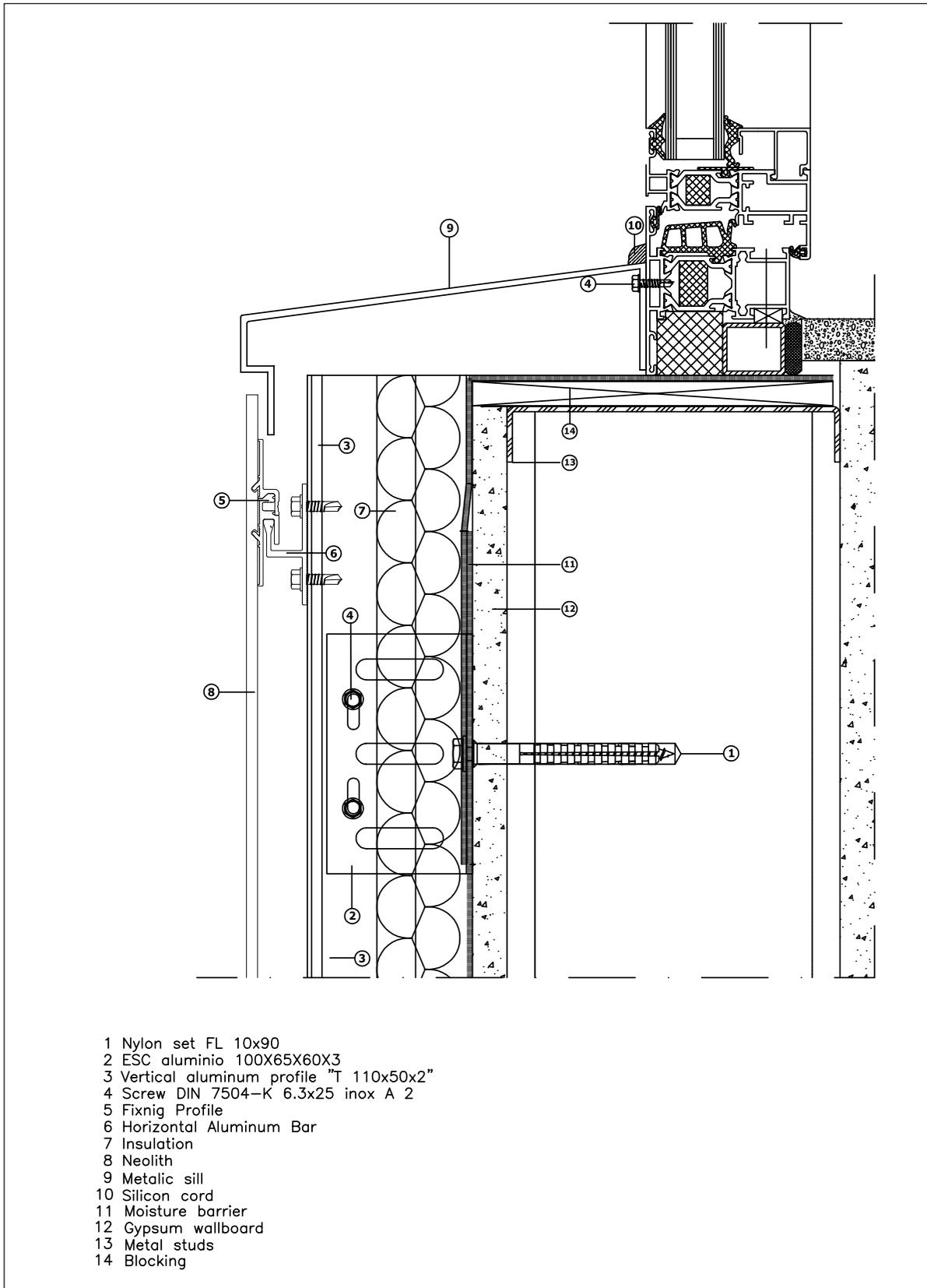
Sill detail. VM system. Vertical section
