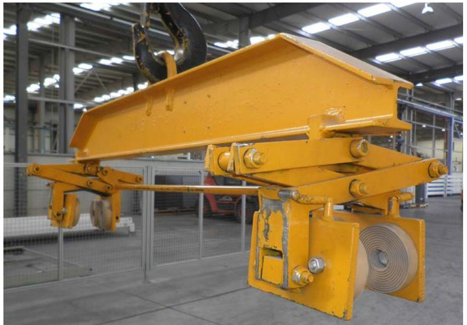
Image 9: Clamp handling for 1/2 mm slabs
