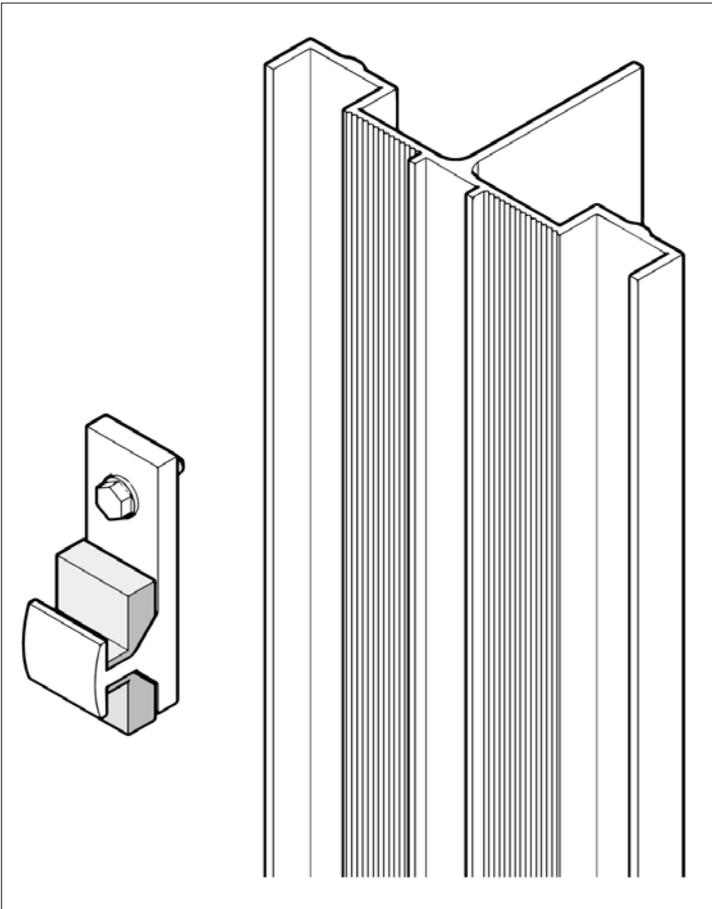
Image 34: Vm System vertical profile and mechanical Clip
