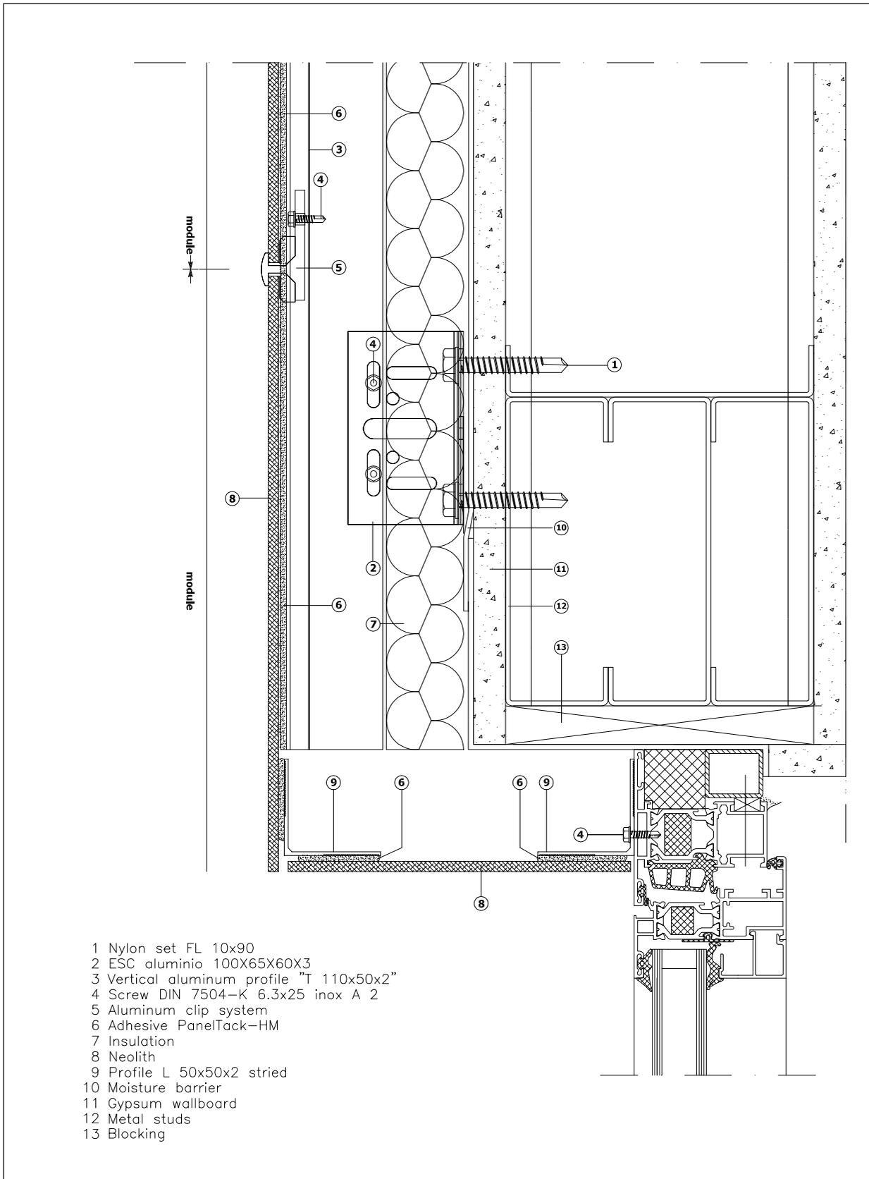
Sill detail. Strongfix system. Vertical section
