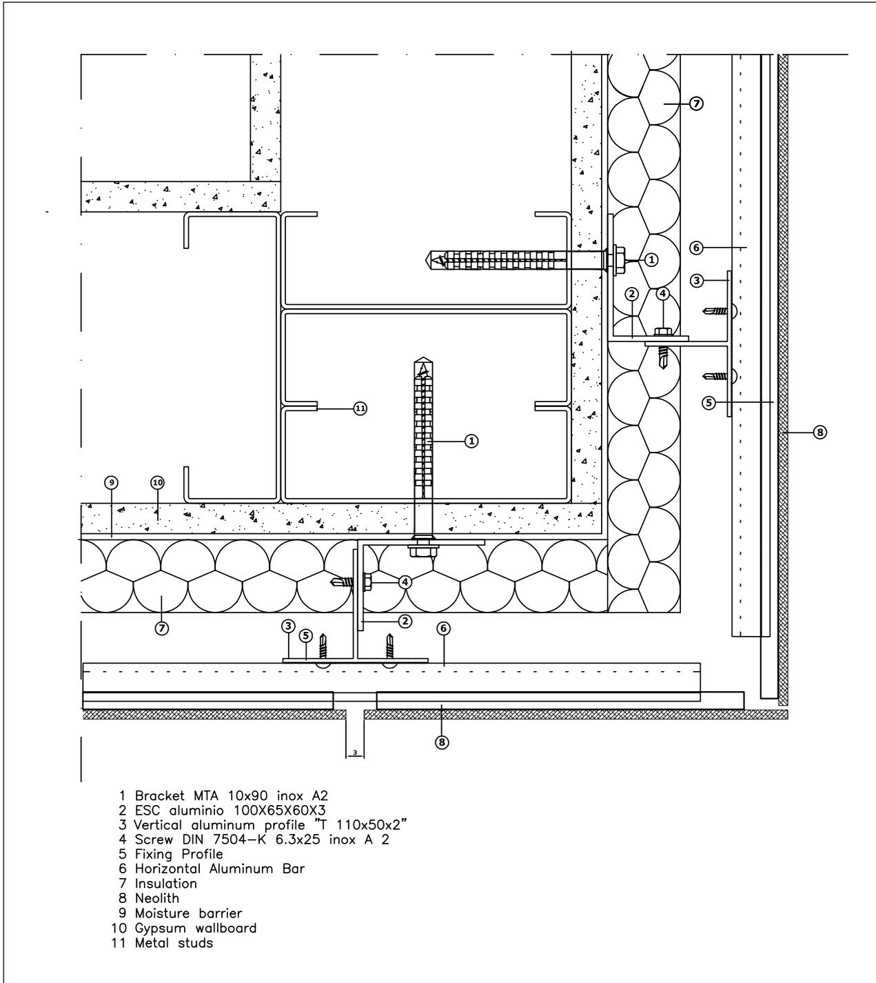
Corner detail. VM system. Horizontal section
